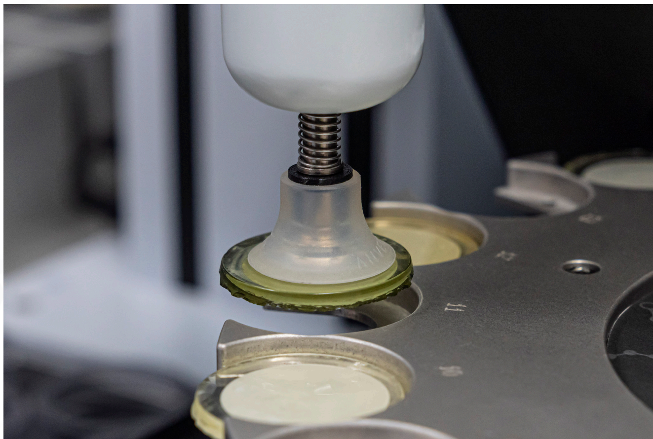
Figure 2. Samples in the carousel ready for analysis, and a sample being delivered from the loading area with the robot arm.
